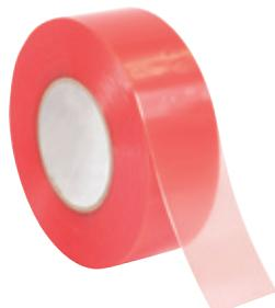
PET double sided tapes with an acrylic, solvent-based pressure sensitive adhesive on both sides.
