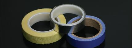
Silicone Glass Tapes are pressure sensitive tapes produced from a silicone rubber coated glass fabric & a high temperature silicone adhesive. The BR1340 is very good at preventing bridging during metalization, and the RR1370 is the most resistant of CFS's silicone rubber coated glass fabric products.
